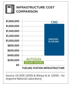
A small, fast-fill CNG station costs approximately \$400,000, according to a 2010 Department of Energy study on the feasibility of natural gas vehicles. Fast-fill dispensers are the preferred option for most fleet and public fueling stations, as they provide similar fill times to gasoline pumps.
